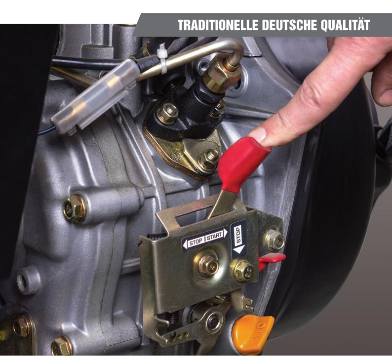
Set the emergency engine switch to START (ON).
